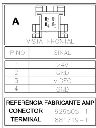
Figura 1.1 – Pin-Out do Conector do Monitor 23”
